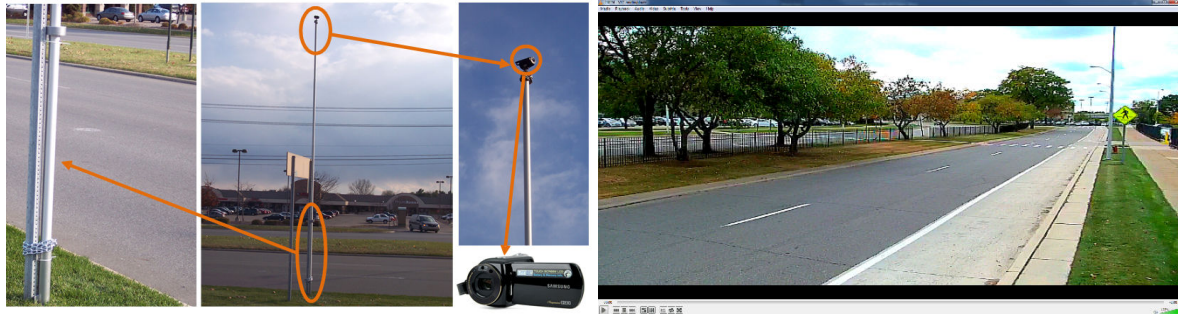
FIGURE 1 Typical video camera setup for recording motorist yielding behavior.
